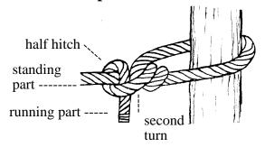
When tied so that the second turn is between the first turn and the standing part ---midshipman's hitch (see direction for midshipman's hitch).
