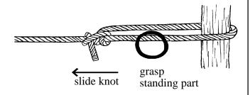
To decrease the tension on a guy line, grasp the standing part just out side the loop, then slid the knot away from your hand.
