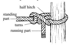
When tied with the two turns outside the loop and the half hitch inside the loop ---- adjustable jam hitch.
