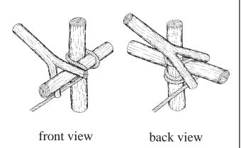
**[STEP 2]** Wrap the rope around the fork of the wrench.
