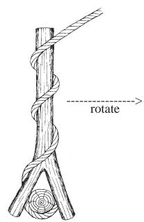
[NOTE] Tighten each turn of a lashing as it is made. The friction between the rope and the pole is too great to tighten more then one turn at a time.
