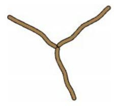
(3) Place the end of one of the unlayed strands under the strand to its left. (Hold the loop open as you work the knot).
