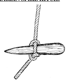
**Description** — A loop formed by a half hitch around a bight in the standing part of the rope.
